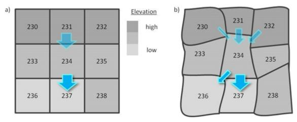
Example grid connections showing water flow between grids. Arrows indicate the water flow in to and out of grid 234, but note that only only water flowing out of each grid is entered in SUEWS\_SiteSelect.txt.
