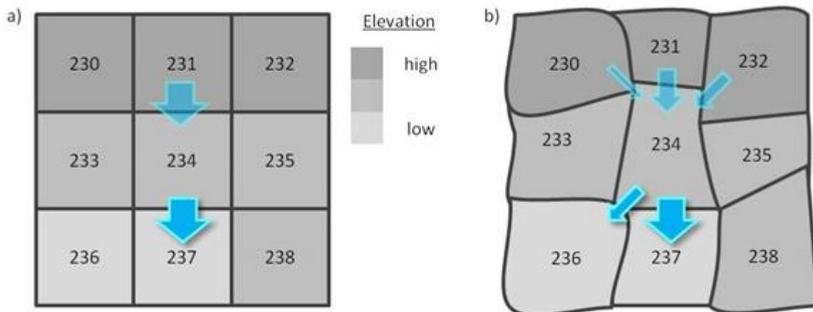
Example grid connections showing water flow between grids. Arrows indicate the water flow in to and out of grid 234, but note that only only water flowing out of each grid is entered in SUEWS\_SiteSelect.txt.
